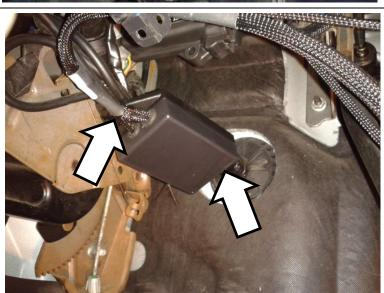
5. Remove the three 5.5mm screws from the bottom of the steering column cover.
