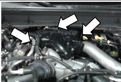
27. Route the MAF connector towards the MAF sensor on the air intake.
