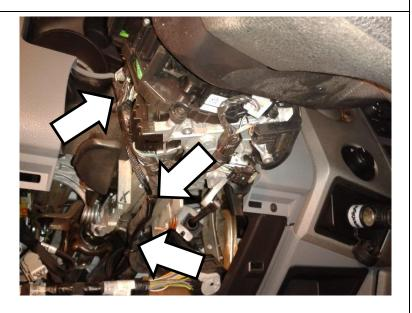
Remove the two 7mm screws securing the OBD connector below the dash.
