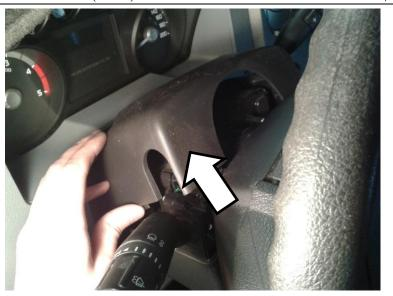
Locate the shift lever connector just behind the hazard lamp switch on the top of the steering column.
