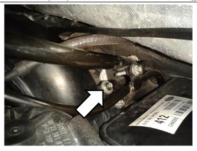
23. Remove the 15 fasteners from the intake manifold. These are 8mm screws. Remove the manifold from the engine.
